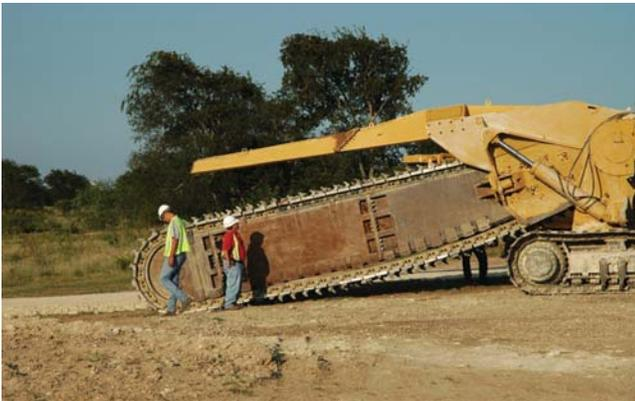
*Trenching Machine Used in Biowall Construction*
